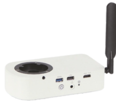
Dovetail mount with built-in 0.43X relay lens
